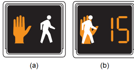
Figure 7.2 – Standard pedestrian signal heads without (a) and with (b) countdown timer
