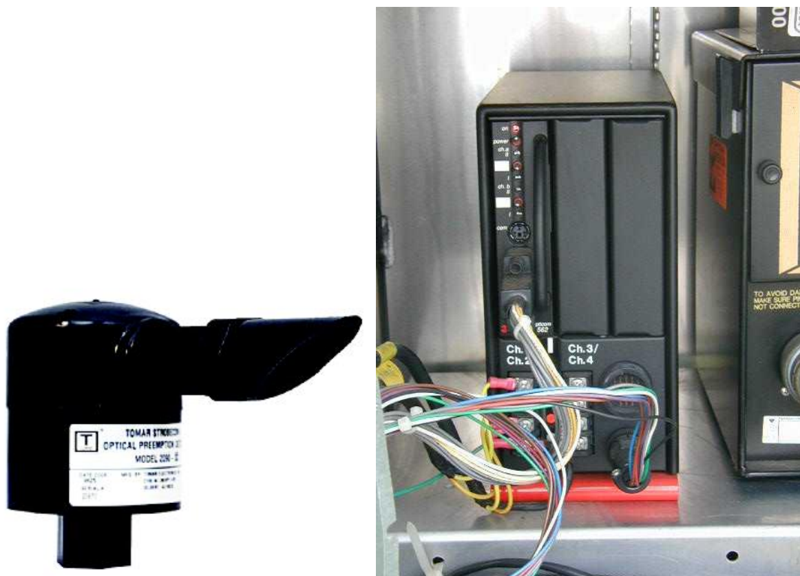
Figure 9.5 – Typical optical pre-emption sensor (left) and phase selector (right)
