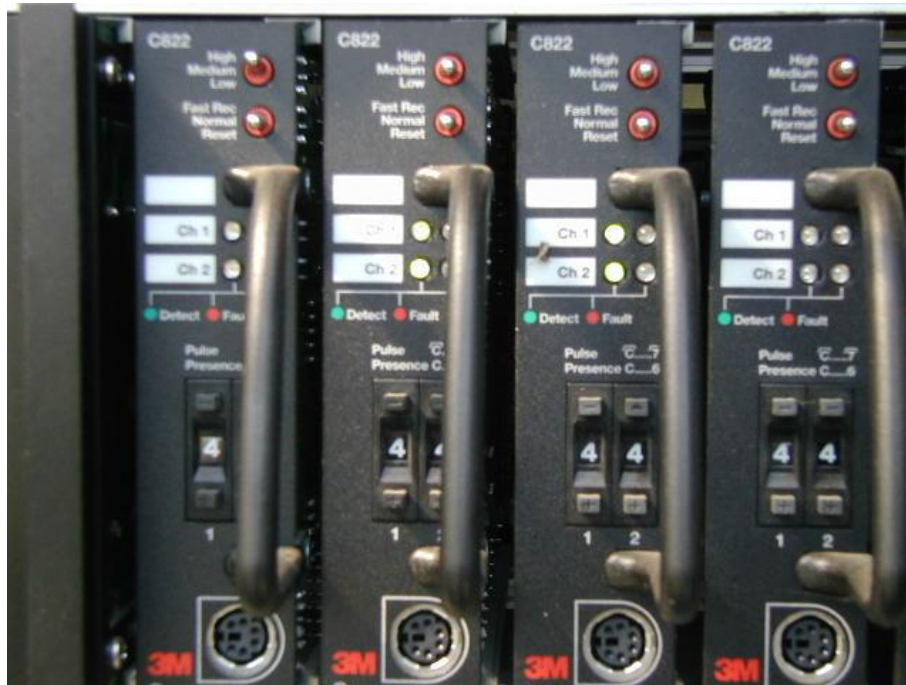
Figure 12.7 – Multi-channel card rack & vehicle loop detectors (2-channel detector/amplifiers shown)
