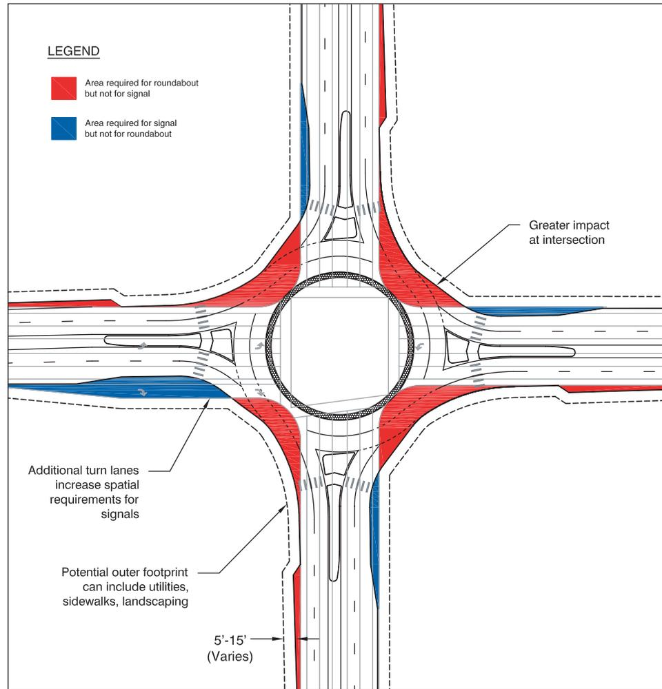
constraints also dictate the need for approach re-alignment to adequately accommodate large semi-trailer combinations while achieving appropriate deflection for small vehicles. In particular, at locations where a WB-67 is anticipated to be the design vehicle, a larger inscribed circle diameter should be planned for when estimating the space requirements of the roundabout.
