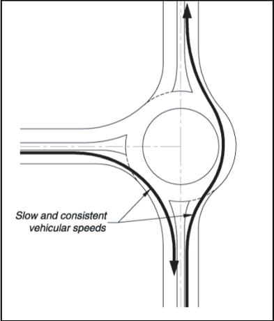
Perpendicular approach angles will generally provide slow and consistent speeds when used in combination with other appropriately sized design features. Achieving acceptable fastest-path speeds is often easier to accomplish with a perpendicular approach angle than with a skew.
