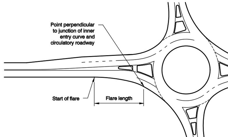
designs. Entry widths should therefore be minimized and flare lengths maximized to achieve the desired capacity with minimal effect on crashes.
