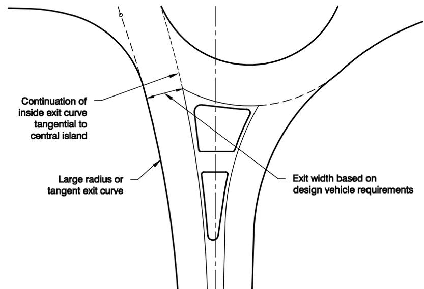
At single-lane roundabouts in urban environments, exits should be designed to enforce slow exit path speeds to maximize safety for pedestrians crossing the exiting traffic stream. Pedestrian activity should be considered at all exits except where separate pedestrian facilities (grade separated paths, etc.) or other restrictions eliminate the likelihood of pedestrian activity in the foreseeable future.
