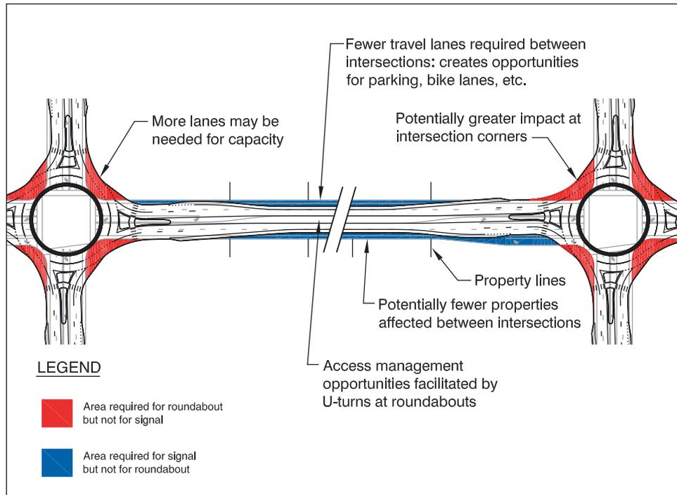
Most roundabouts on arterial streets are designed to accommodate traffic volume estimated for a future horizon year, which can extend 20 years or more from the construction date. Collector and local-street roundabouts are typically designed for full build-out conditions. While it is important to plan for future traffic volume and capacity needs, the immediate effects on pedestrian and bicycle users should also be considered. A roundabout constructed with a wide
