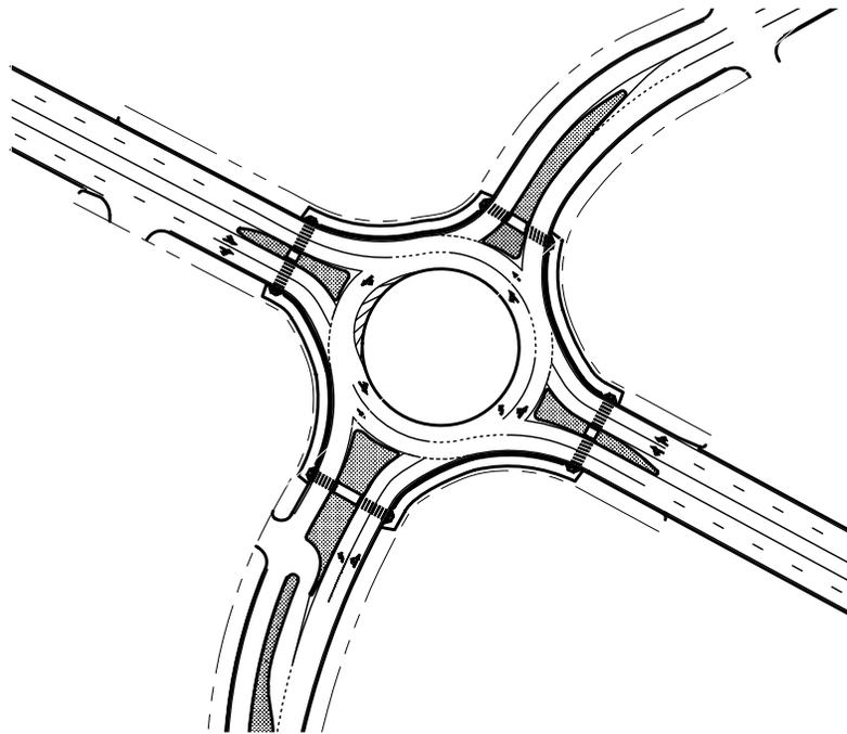
(b) Staged Multilane Roundabout: Ultimate Configuration
