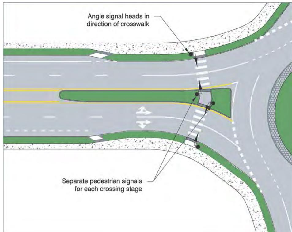
The second, more definitive method to resolve the concerns above is to offset the two crosswalks by providing a staggered walkway within the splitter island, as shown in Exhibit 7-31. The offset clearly indicates to pedestrians that there are two separate stages to the pedestrian signal, and it moves the pedestrian signal heads away from each other so that pedestrians will not be likely to observe the
