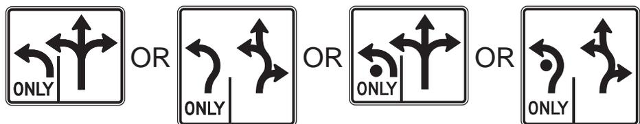
of the lane-control signs adjacent to the corresponding lane-use arrow markings. An optional second set of lane designation signing (not shown in Exhibit 7-20) may also be provided upstream of the pedestrian crossing, adjacent to the second set of lane-use arrow markings. The redundant lane-use signing may help to reinforce the lane-use messages to drivers, particularly for more complex lane configurations. Any additional signs should be balanced against the concern for creating sign clutter.
