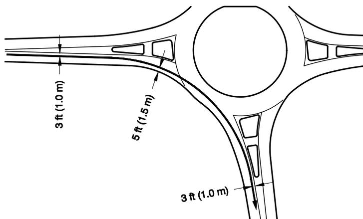
then measure the minimum radii using suitable curve templates or by replicating the path in CAD and using it to determine the radii. The Wisconsin Department of Transportation *Roundabout Guide* (7) provides one possible technique for creating fastest paths in CAD.
