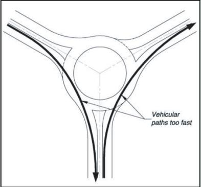
In situations involving a large angle between legs, it is desirable to realign one or more legs to try to achieve a more perpendicular condition. Large angles make it difficult to provide adequate deflection and may result in fast vehicle speeds, particularly for the right-turn movements.
