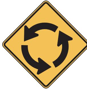
users that they are approaching an intersection with the form of a roundabout. This sign, introduced in the 2003 edition of the MUTCD, has many advantages over advance warning signs that have been used at roundabouts in the past:
