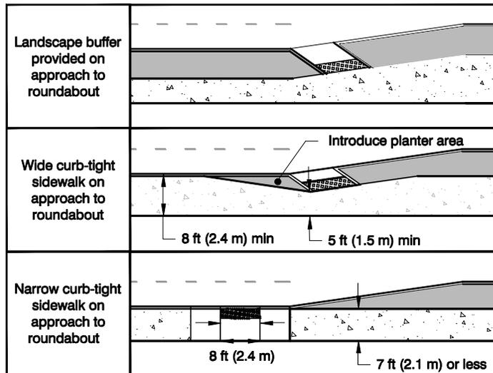
Since bike ramps can be confusing for pedestrians with vision impairments, detectable warnings should be included on the ramp. Where the ramp is placed in a planter strip, the detectable warning field should be placed at the top of the ramp since the ramp itself is part of the vehicular area for which the detectable warning is used. If the ramp is in the sidewalk itself, the detectable warning should be placed at the bottom of the ramp. Other aspects of the bike ramp design and placement can
