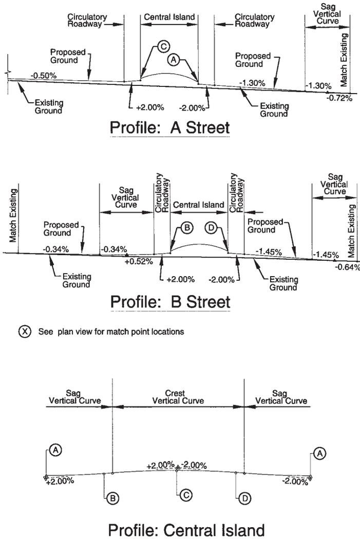
may also be beneficial to the engineer, reviewers, and contractor. The combination of the central island, inscribed circle, and curb profiles allows for quick verification of cross slopes and drainage and provides additional information to contractors for staking out the roundabout.
