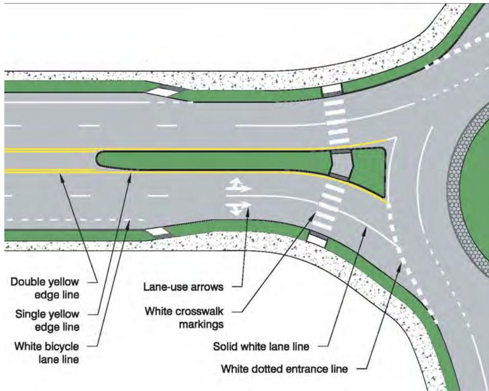
double yellow lines. For small splitter islands [area less than 75 ft<sup>2</sup> (7 m<sup>2</sup>)], the island may consist of pavement markings only, in the form of two sets of double yellow lines or marking the entire splitter island yellow. However, raised splitter islands should be used where possible.
